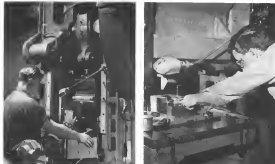
ROLLING OPERATIONS on T58 compressor blades are performed by friction in 55-ton press (left). Plates are hydraulically opened to position and hold blade during rolling. Follow-up operation (right) shows blade placed in cooling die to provide initial contour.
